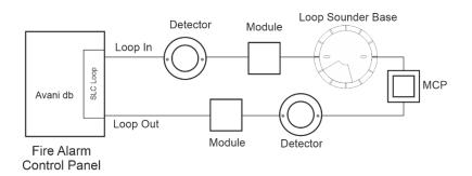
Connect the Loop Positive & Negative wires to SLC IN Terminal, observing the polarity. The wiring Terminal accepts solid or stranded cables up to 2.5 mm<sup>2</sup>.
